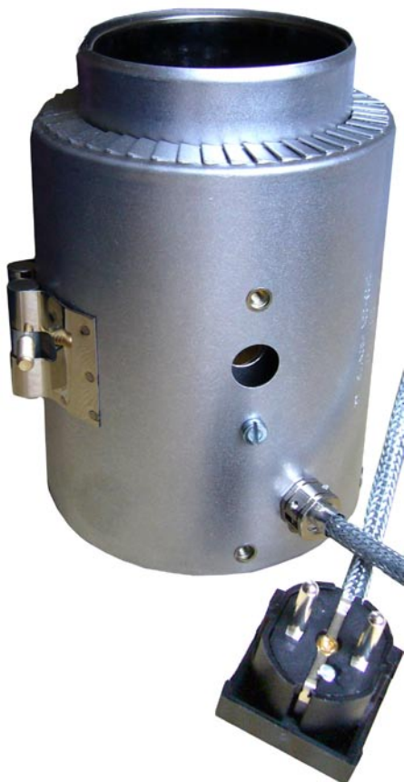
ZH206, \varnothing 80 x 175mm, 1750W, 230V, kabel A=800, konektor Schuko, pro Arburg, obj.č. 39000253, ZH06-00X
